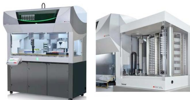
*Figure 1: The Fluent cell-based assay workstation. A Fluent 780 is shown, equipped with an eight-channel Flexible Channel Arm, a Multiple Channel Arm 384 and a Robotic Gripper Arm. A Carousel is integrated onto the right hand side of the instrument, along with the latest generation of CO<sub>2</sub> incubator. An Infinite M1000 PRO microplate reader is located below the Dynamic Deck. The instrument was also equipped with a HEPA hood (not shown).*
