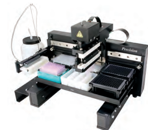
Figure 4 – Precision™ Microplate Pipetting System is an affordable, innovative solution for automated 96-/384-well microplate liquid handling. The unique XY transport design provides effortless 96- to 384-well plate transfers with the same pipette mechanism. The instrument was used to serially titrate enzyme as well as inhibitor across a 96-well plate, as well as transfer the to the 384-well assay plates
