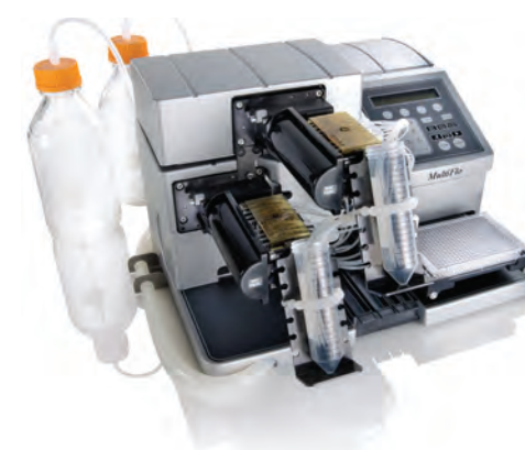
Figure 3 – MultiFlo™ Microplate Dispenser offers up to four reagents dispensed in parallel with one compact instrument. The MultiFlo offers a choice of either peristaltic pump or microprocessor controlled syringe drive technologies. A wide array of plate types are accommodated from 6- to 1536-well formats as well as a broad volume range from 1 μL to 3 mL. The peristaltic pump cassettes consist of 8 individual tubes allowing for dispensing of a range of different reagents across the channels.
