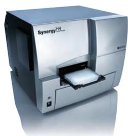
**Figure 3** – Synergy<sup>™</sup> H4 Hybrid Multi-Mode Microplate Reader combines a filter-based and monochromator-based detection system in one unit. The HTRF<sup>®</sup> certified reader uses the filter-based system and Xenon flash lamp to detect the 665 nm and 620 nm fluorescent emissions from this chemistry using Ex: 330/80 nm; Em: 620/10 and 665/8 nm filters, and a 365 nm cutoff dichroic mirror.
