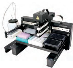
**Figure 1** – Precision<sup>™</sup> Microplate Pipetting System combines an 8-channel pipetting head and an 8-channel bulk reagent dispenser in one instrument. The instrument was used to perform the serial dilutions of test antibodies and binding proteins, and transfer aliquots into the LV384-well assay plates.
