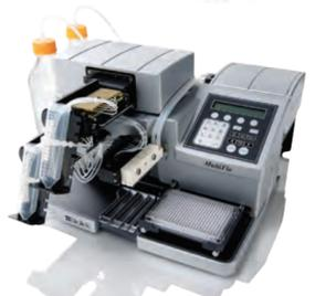
**Figure 2** – MultiFlo<sup>™</sup> Microplate Dispenser offers fast, accurate plate dispensing capabilities through its two peristaltic and two syringe pumps, with volumes ranging from 1-3000 µL. The instrument was used to dispense cryopreserved cells, media, EC<sub>50</sub> concentrations of test antibodies, as well as labeled acceptor antibodies.
