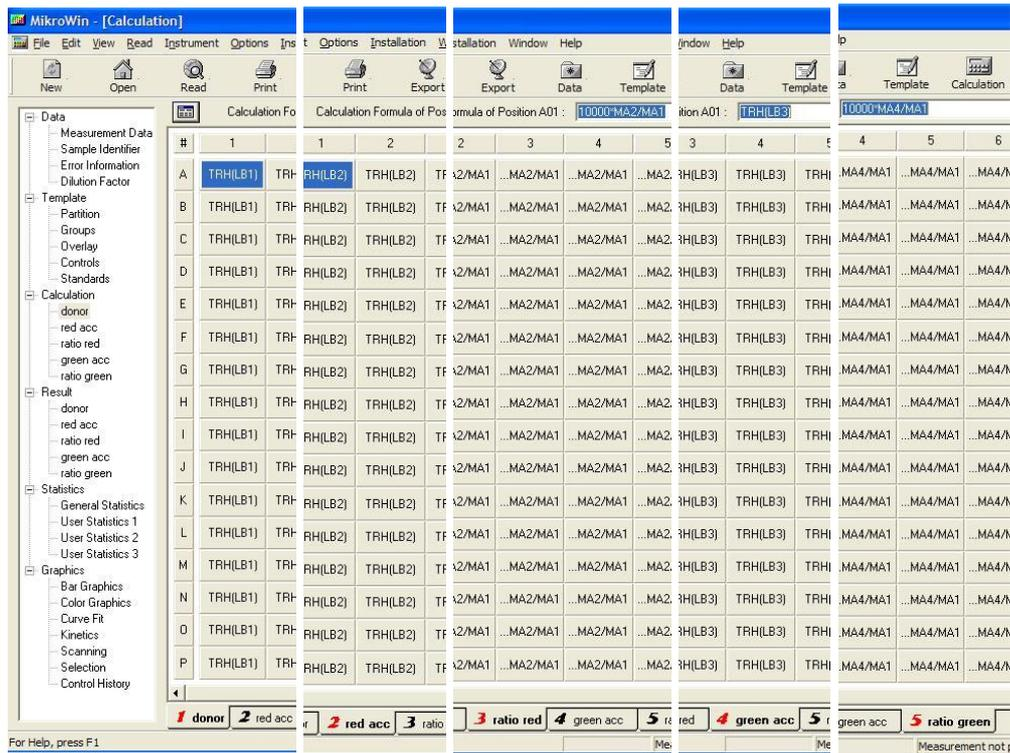
**Figure 4c.** Instrument settings for HTplex™. *Calculation Matrices* holding the individual readings and the calculations of the red and the green ratios for each well. Each of the matrices can be selected for data export into spreadsheet or data base software.
