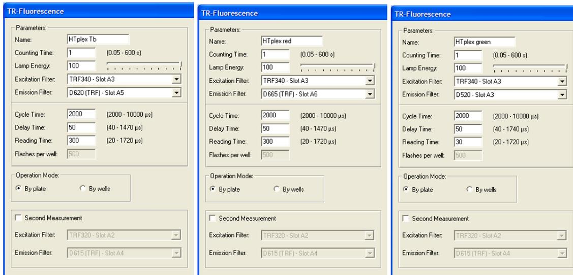
**Figure 4b.** Instrument settings for HTplex™. **Operations** dialogues with filter and timing definitions for the 3 sequential measurements of donor, red acceptor and green acceptor.
