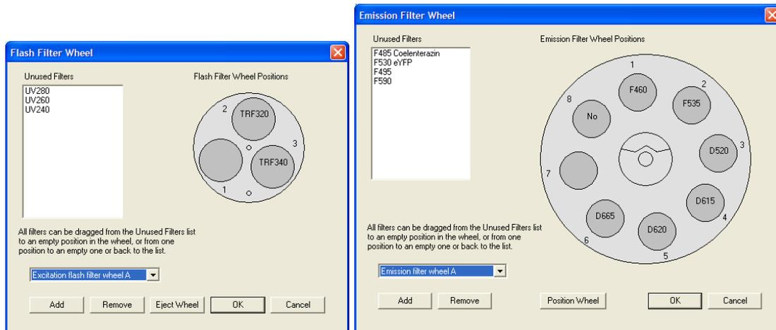
**Figure 4a.** Instrument settings for HTplex™. Global definition of the optimum excitation filter **TRF340** for Tb cryptates and the emission filters **D520**, **D620** and **D665** for the specific emission spectra of donor and acceptors.
