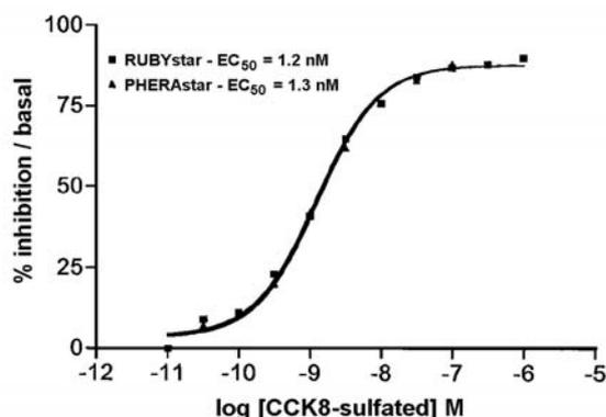
**Fig. 3:** Direct performance comparison of the PHERAstar with the RUBYstar using the HTRF® IP-One assay. The 1321N1-CCK1 cell line and CCK8-sulfated as agonist were applied.
