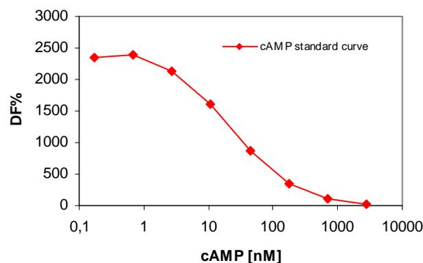
**Figure 1:** HTRF<sup>®</sup> cAMP calibration curve measured on the Safire<sup>2™</sup> after 1 h of incubation using white 384-well plates (Greiner<sup>®</sup>). EC<sub>50</sub> = 24 nM;  $z'$  = 0.74
